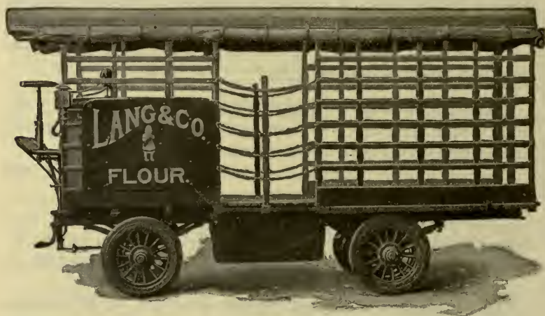
FIG. 407.—Heavy truck of the Vehicle Equipment Co. Carrying capacity, 4 tons; speed, 6 miles per hour; travel radius on one charge of battery, 25 miles.
